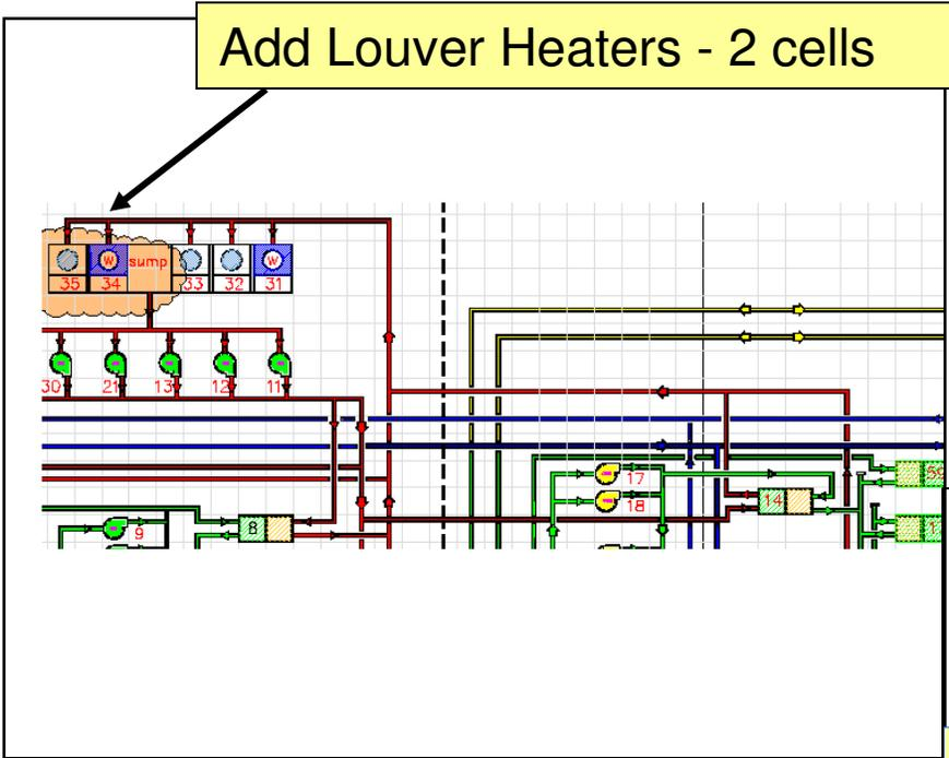
Install pumps, piping and controls into existing louver heater piping
